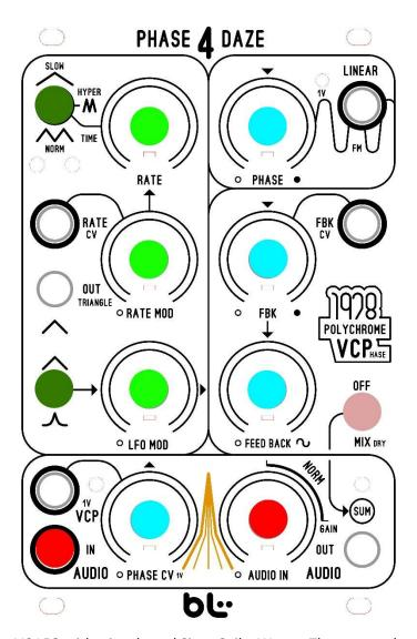
**Section Green**. Analog VC LFO with triangle and Sinus Spike Waves. The top toggle switch controls the range of the Ifo. Hyper is for audio rate modulation, norm is for the original Ifo speed, and slow is for really slow Ifo modulation.
